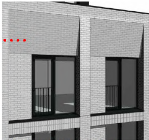
Brick soffit detail to Ellesmere Street Elevation
